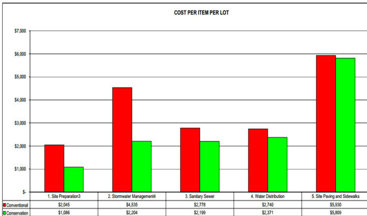
Figure 3 – Cost Breakdown for Each Aspect of Lot Development – Mill Creek vs. Sunset Prairie
